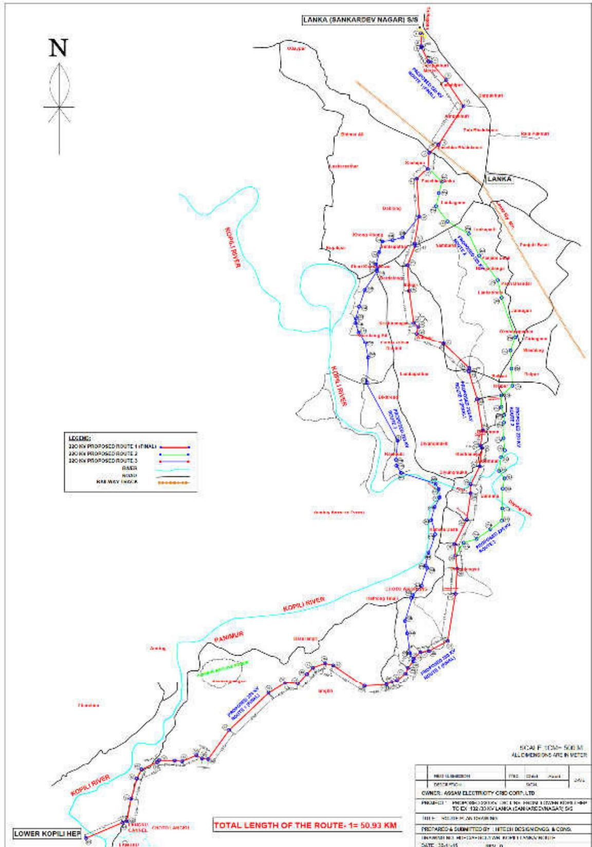
Figure 4: Proposed route map on Topographical sheet for the 220 kV TL
