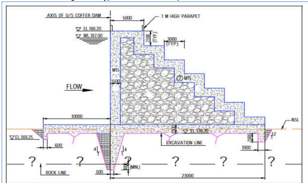
Figure 16: Typical Section of the Downstream Cofferdam
