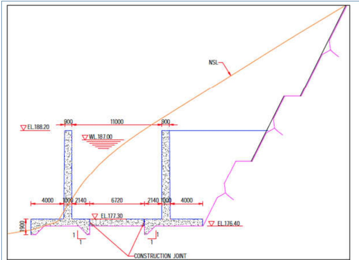
Figure 14: Dam Section through Spillway Sluice
