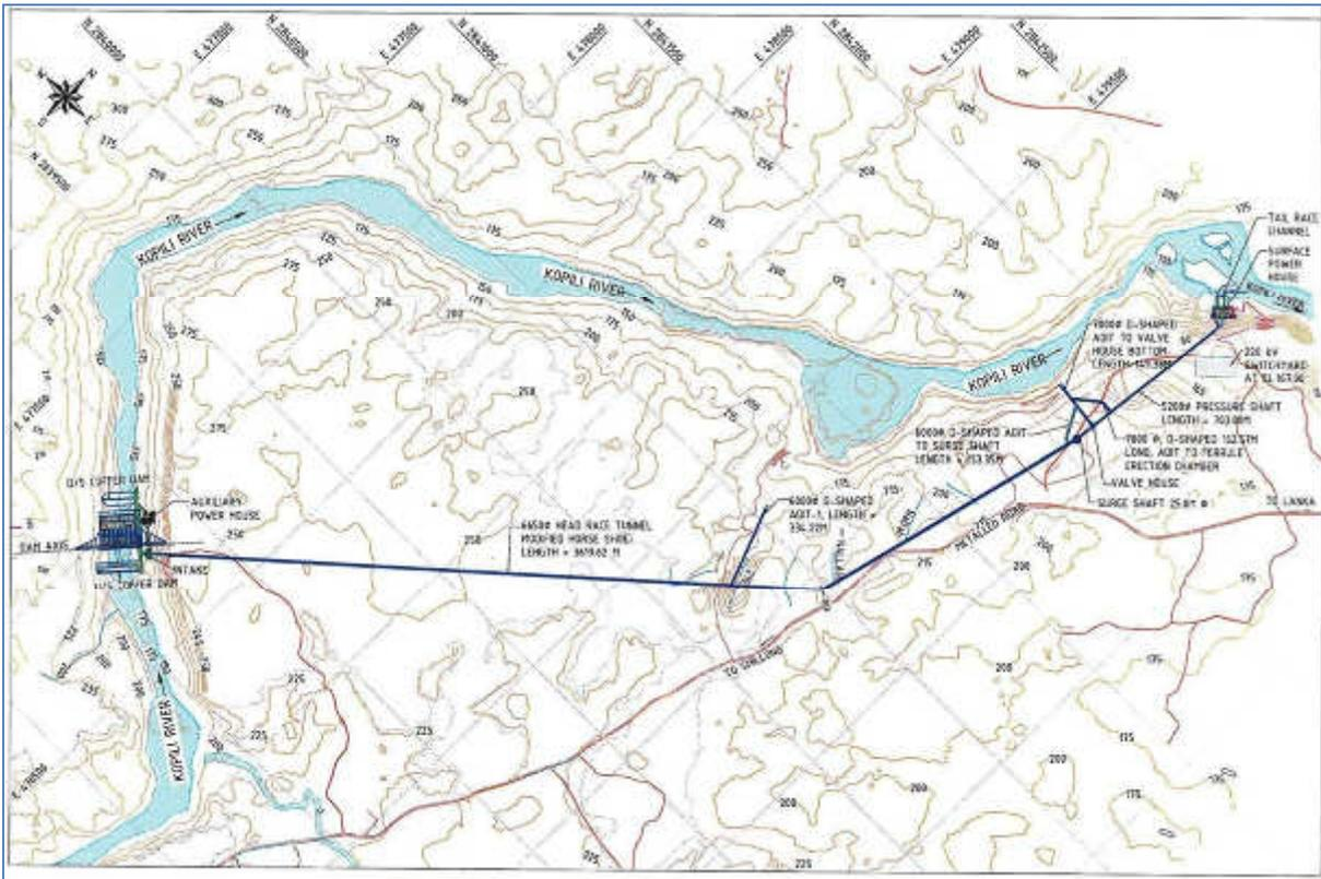
Figure 8: Proposed route map on Topographical sheet for the 220 kV TL
