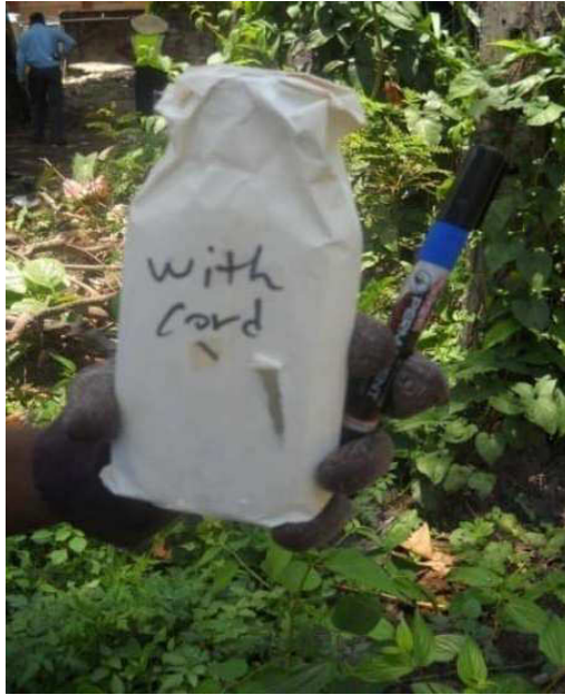
Fig. 4 - Sterilized sample bottle used for the collection of water samples for bacteriological analysis
