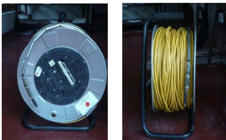
Fig. 3 : Front view and side view of Dip meter
