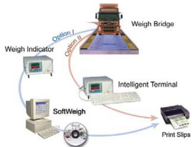
Picture 8 Typical weigh bridge system
