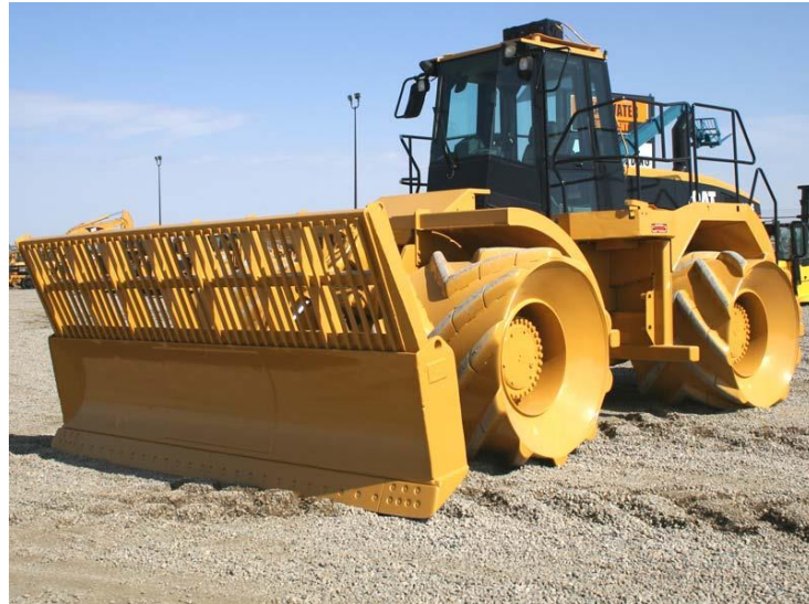
Picture 9 Waste Compactor
