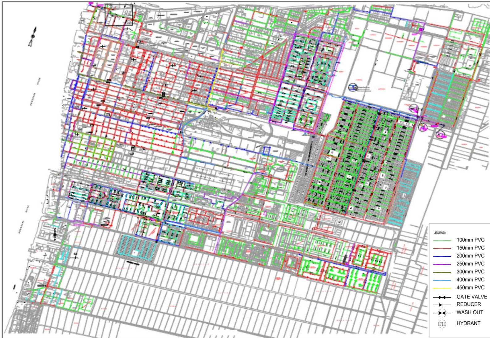
Figure 2.5: Georgetown Component - System Distribution Network
