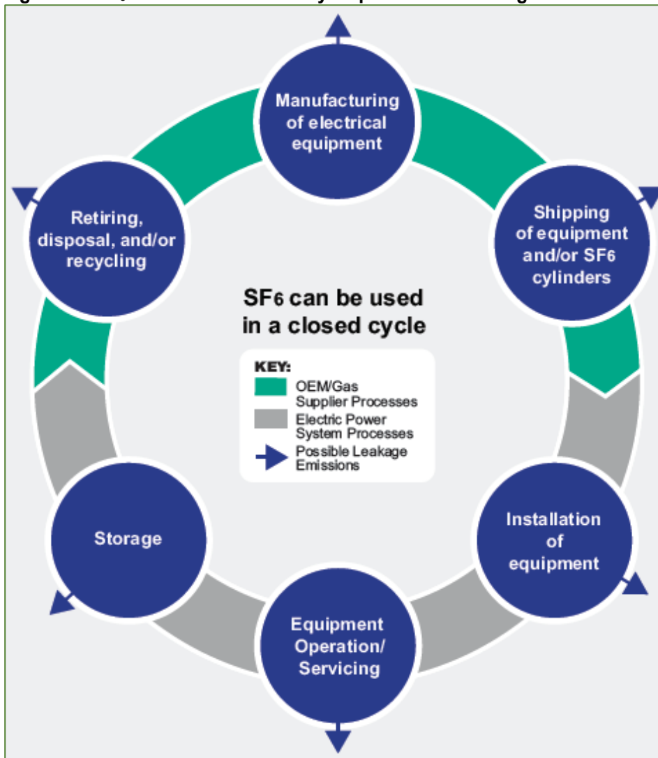
Figure 23. SF 6 emissions in the lifecycle process of switchgear
