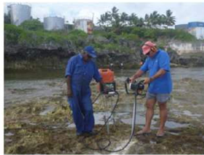
Plate 3: Drilling Borehole –NU 15 on the crest of the fringing reef Alofi.
