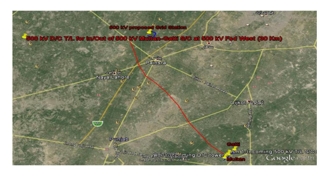
Figure 1.2: Site of proposed 500 KV D/C T. Line for In/Out of 500 kV Multan-Gatti S/C At 500 kV Faisalabad West Grid Station
