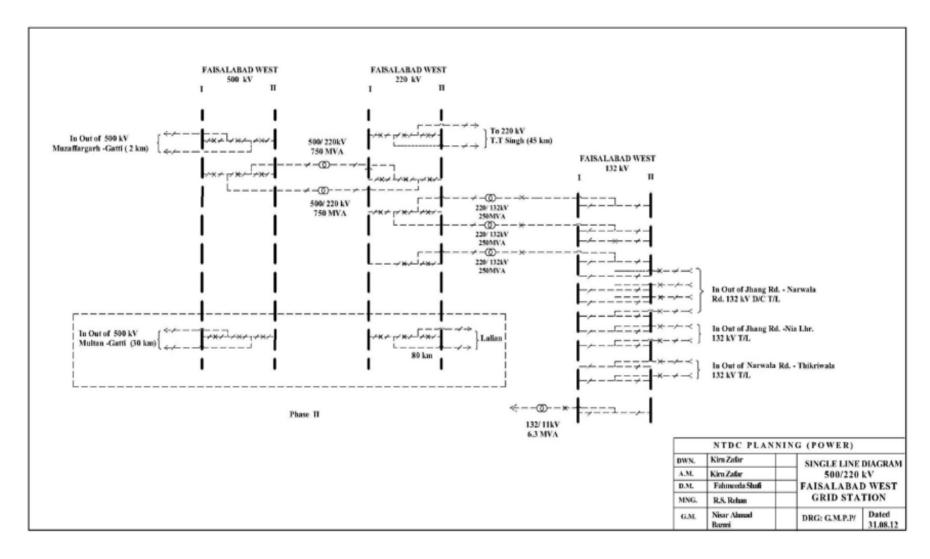
Fig 2.3: Single Line Diagram 500/220 Faisalabad West Grid Station
