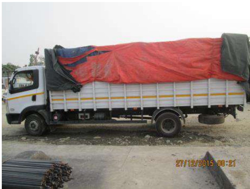
Photograph 9: Trucks are being covered with Tarpaulin while transporting the material (AH-02)
