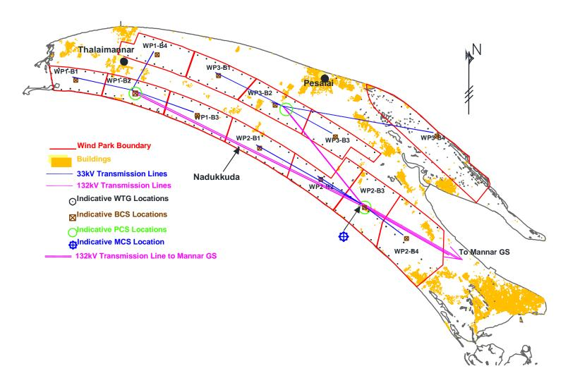
Note: Transmission layout is conceptual, and line routes and substation locations are to be defined more accurately during the feasibility study.
