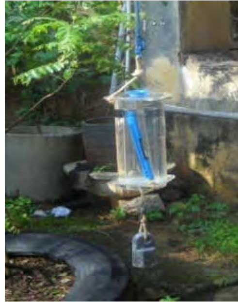
Fig. 5 – Depth sampler used for the collection of groundwater samples from wells
