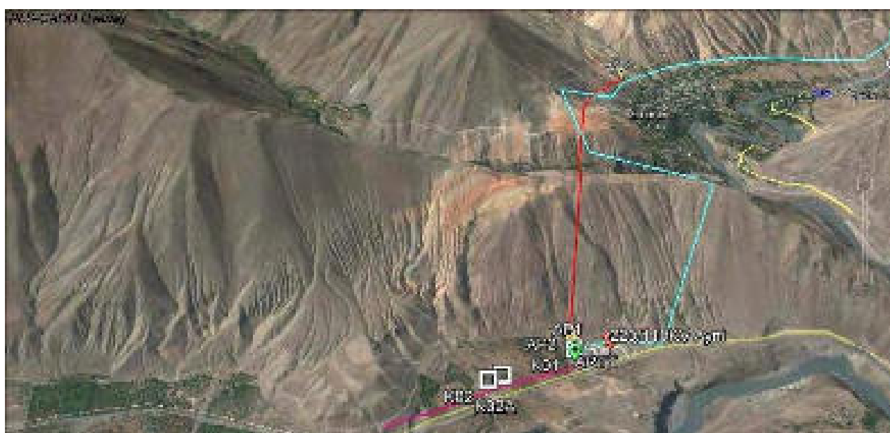
Ayni Substation; Old (light blue) and new (red) OHL proposal, existing line is presented in violet
