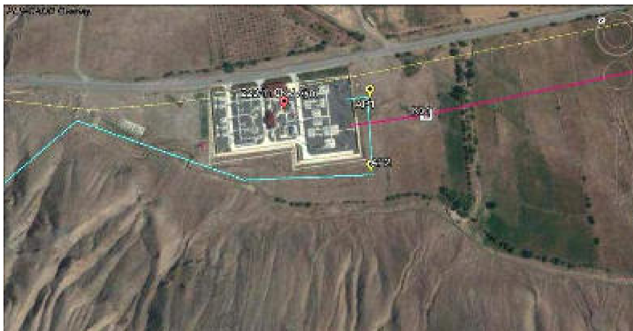
Ayni Substation; Old proposal, new OHL (light blue) crossing existing line (violet)
