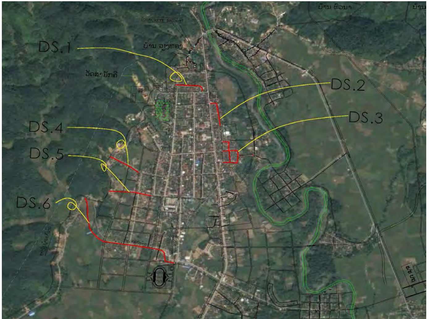
Figure 14. Road drains to be upgraded in Luang Namtha
