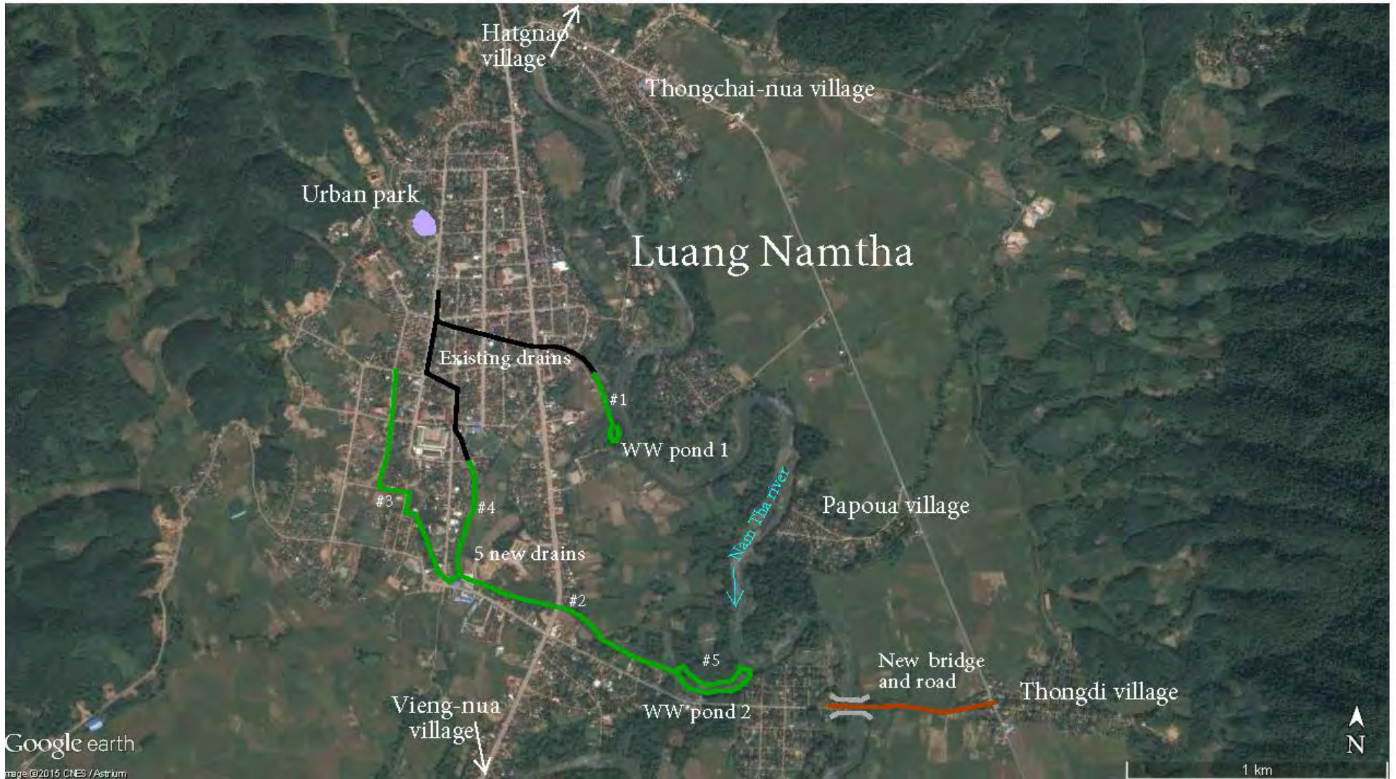
Figure 12. Demonstration villages, WW ponds & drains, and new road & bridge
