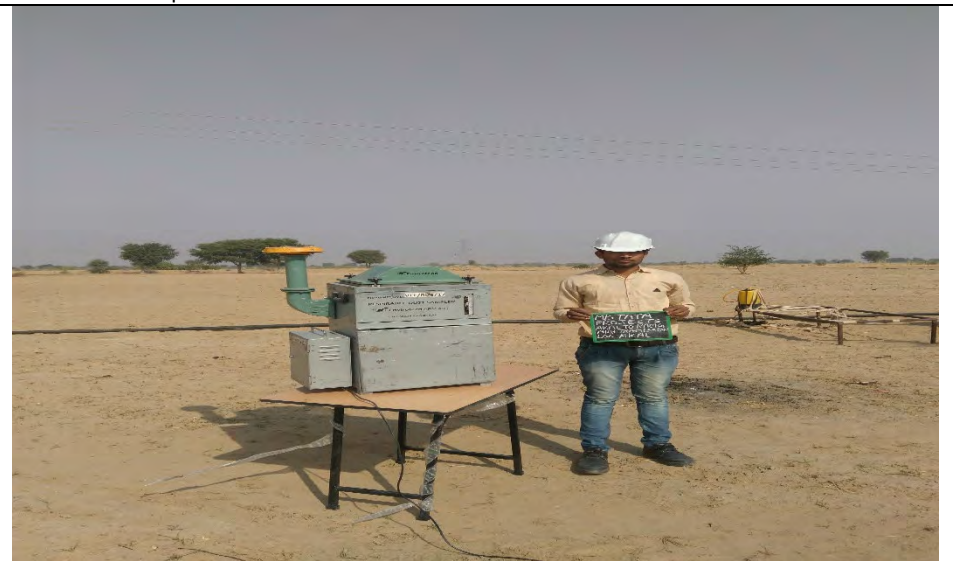
1.12 Air Sample RDS collection at Site
