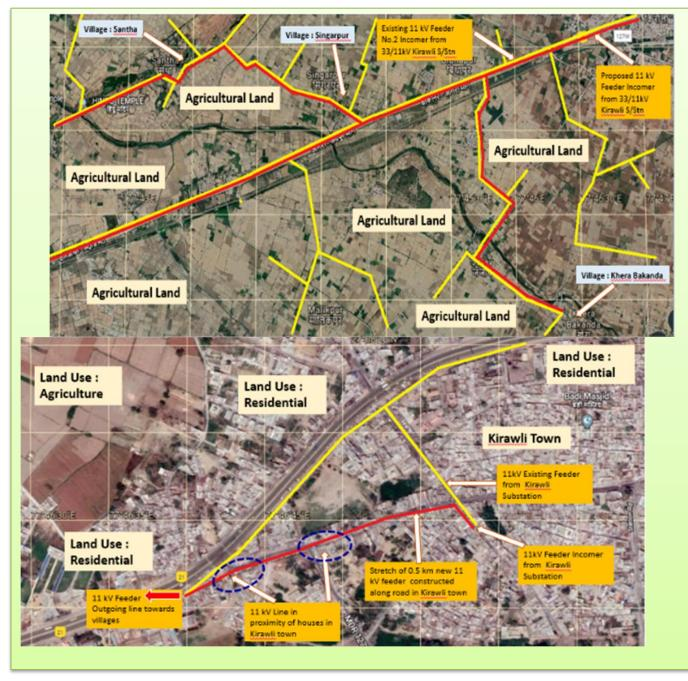
Figure 5: Feeder No 2 (incomer from 33/11 kV Kirawli substation) in PVVNL
