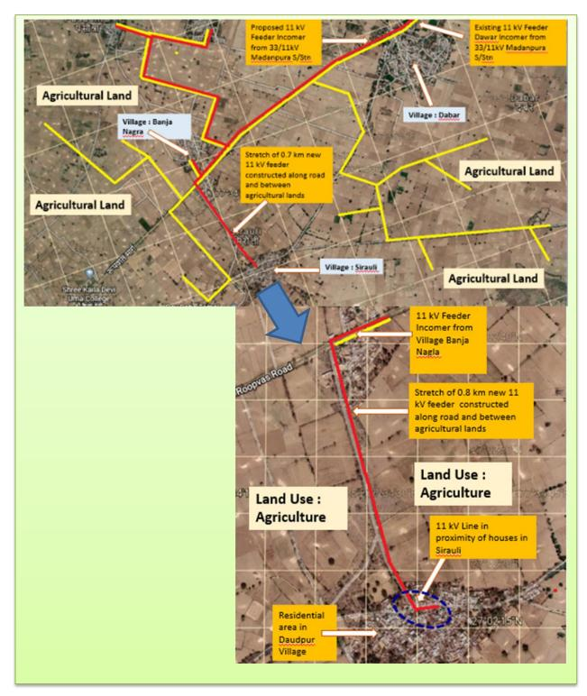
Figure 4: Dawar Feeder (incomer from 33/11 kV Madanpura substation) in PVVNL
