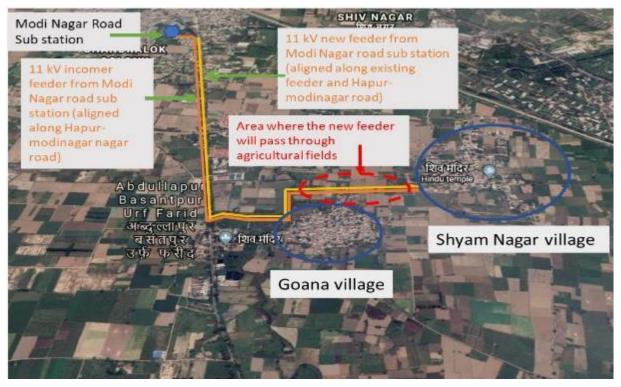
Figure 8: Goana Shyam Nagar Feeder (incomer from 33/11 kV Modinagar Road Substation) in Bulandshahar Zone in DVVNL
