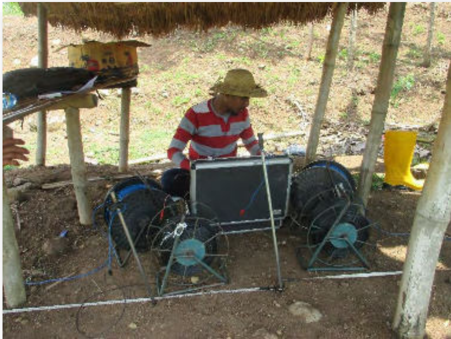
Geoelectrical investigation process
