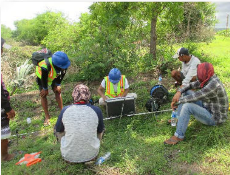
Geoelectrical investigation process
