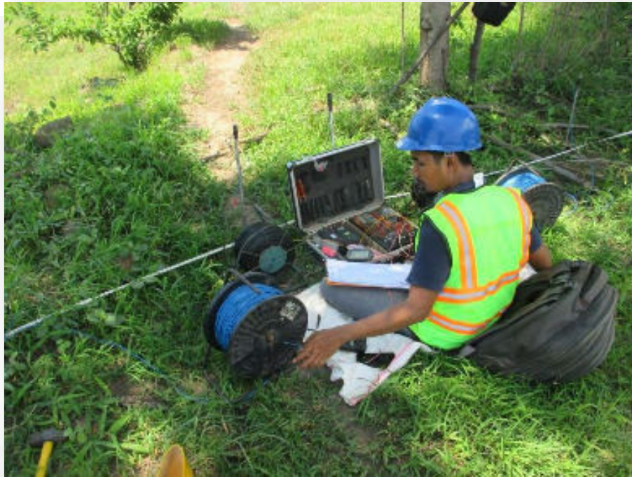
Geoelectrical investigation process
