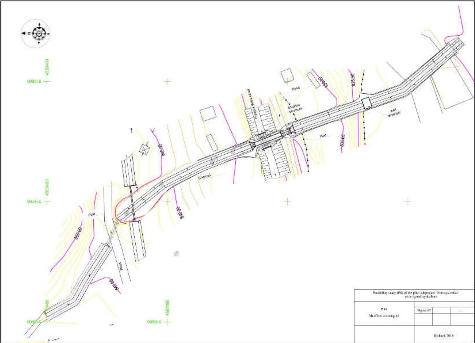
Figure 8: Horizontal alignment of the future mudflow crossing structure over the Pravaya-Vetka canal on km 15+25
