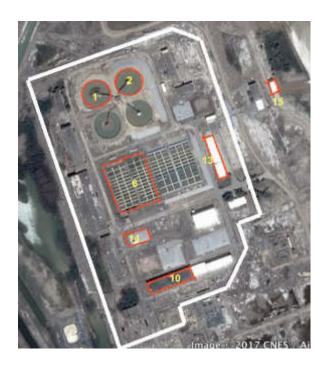
**Picture 41:** Project works at Takhiatash WTP (circled in red) rehabilitation of: circular clarifiers -1, 2; filtration facilities – 6; 1<sup>st</sup> lift pumping station – 15, 2<sup>nd</sup> lift pumping station – 10, mixing chamber - 13
