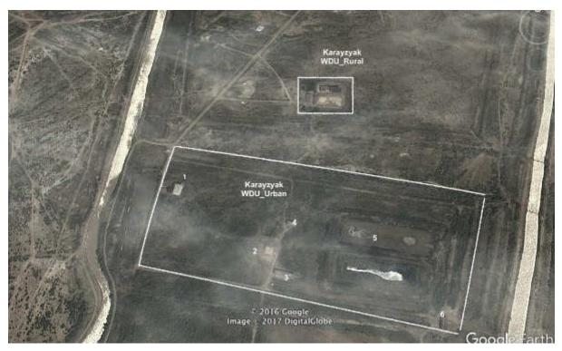
**Picture 21:** Urban and rural WDCs in Karauzyak district. For urban WDC – 1-administrative building/laboratory, 2 – CWR, 3 - 2<sup>nd</sup> lift pumping station, 5 – sedimentation ponds (not operational now), 6 – 1<sup>st</sup> lift pumping station (not operational)
