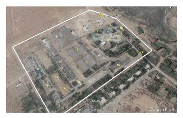
**Picture 4:** Layout of Tuyamuyun WTP (1-4 circular clarifiers, 5-6 longitudinal clarifiers, 7-8 filtration facilities, 9-11 Clean Water Reservoirs, 12 – 2<sup>nd</sup> lift pumping station, 13 – pumping station for own needs, 14-administration, laboratory, 15 – reagent unit, 16 – chlorination unit, 17-entrance)
