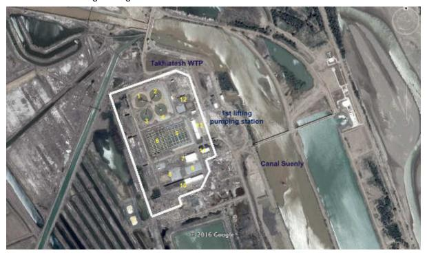
**Picture 6:** Layout of Takhiatash WTP (1-4 circular clarifiers, 5-6 longitudinal clarifiers, 7 filtration facilities, 8-9 Clean Water Reservoirs, 10 – 2<sup>nd</sup> lift pumping station, 11-administration, laboratory, 12 – chlorination unit, 13 – reagent unit)
