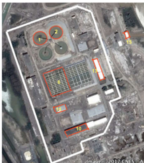
Picture 41: Project works at Takhiatash WTP (circled in red) rehabilitation of: circular clarifiers -1, 2; filtration facilities – 6; 1 st lift pumping station – 15, 2 nd lift pumping station – 10, mixing chamber - 13
