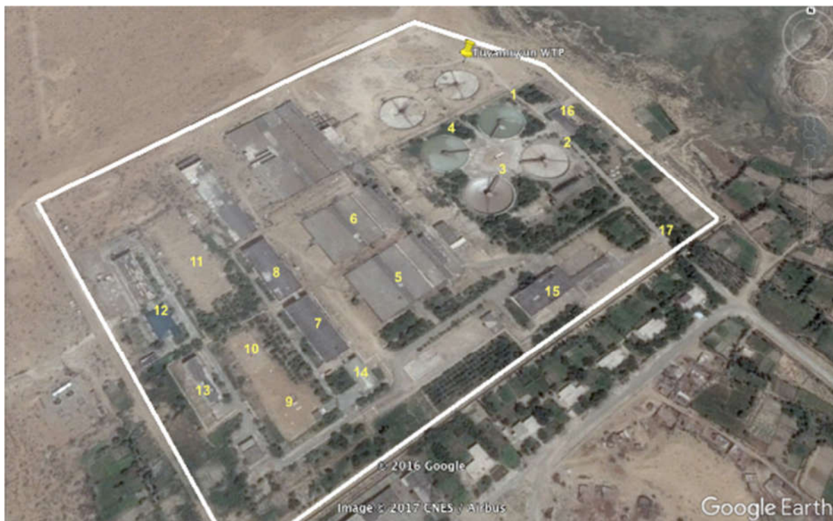
Picture 4: Layout of Tuyamuyun WTP (1-4 circular clarifiers, 5-6 longitudinal clarifiers, 7-8 filtration facilities, 9-11 Clean Water Reservoirs, 12 – 2 nd lift pumping station, 13 – pumping station for own needs, 14-administration, laboratory, 15 – reagent unit, 16 – chlorination unit, 17-entrance)
