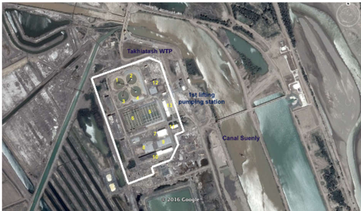
Picture 6: Layout of Takhiatash WTP (1-4 circular clarifiers, 5-6 longitudinal clarifiers, 7 filtration facilities, 8-9 Clean Water Reservoirs, 10 – 2 nd lift pumping station, 11-administration, laboratory, 12 – chlorination unit, 13 – reagent unit)
