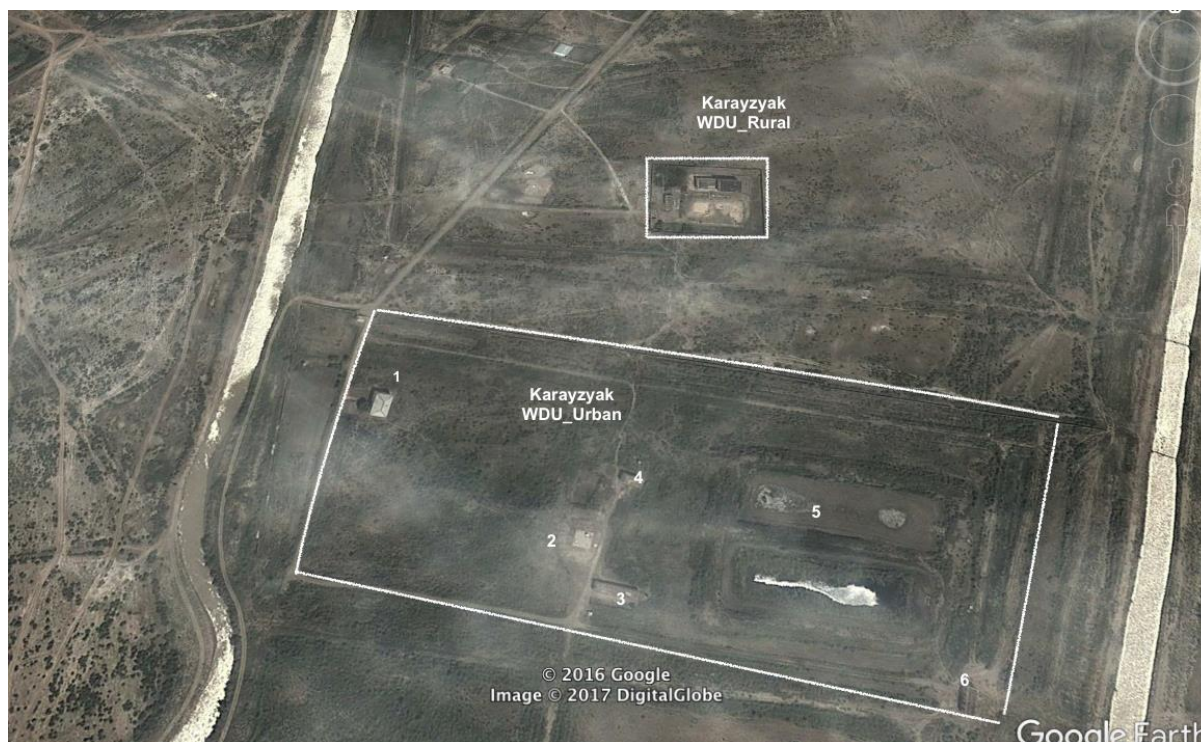
Picture 21: Urban and rural WDCs in Karauzyak district. For urban WDC – 1-administrative building/laboratory, 2 – CWR, 3 - 2 nd lift pumping station, 5 – sedimentation ponds (not operational now), 6 – 1 st lift pumping station (not operational)
