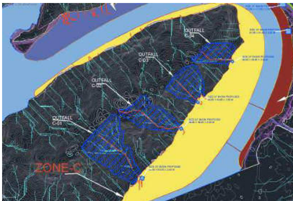
Fig. 2.4 The above diagram shows the pond sizes that have been arrived for the major outfalls of Zones C
