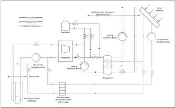
Figure 31: GSHP system schematic.
