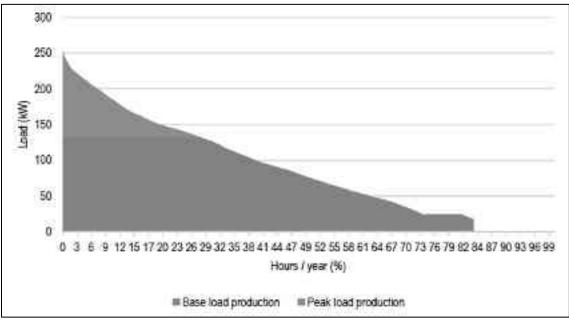
Figure 29: Preferred capacity mix for the GSHP system.
