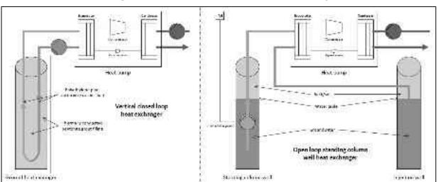
Figure 83: Closed and open loop heat exchangers.
