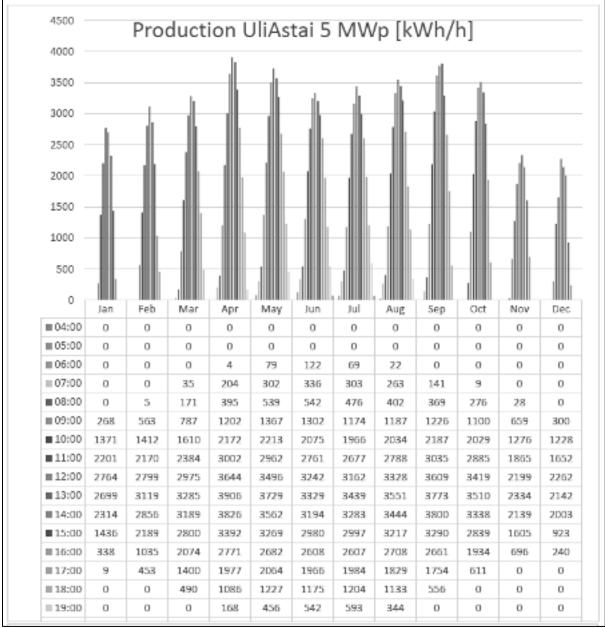
Figure 10: Uliastai solar PV farm estimated production (kWh/hr).
