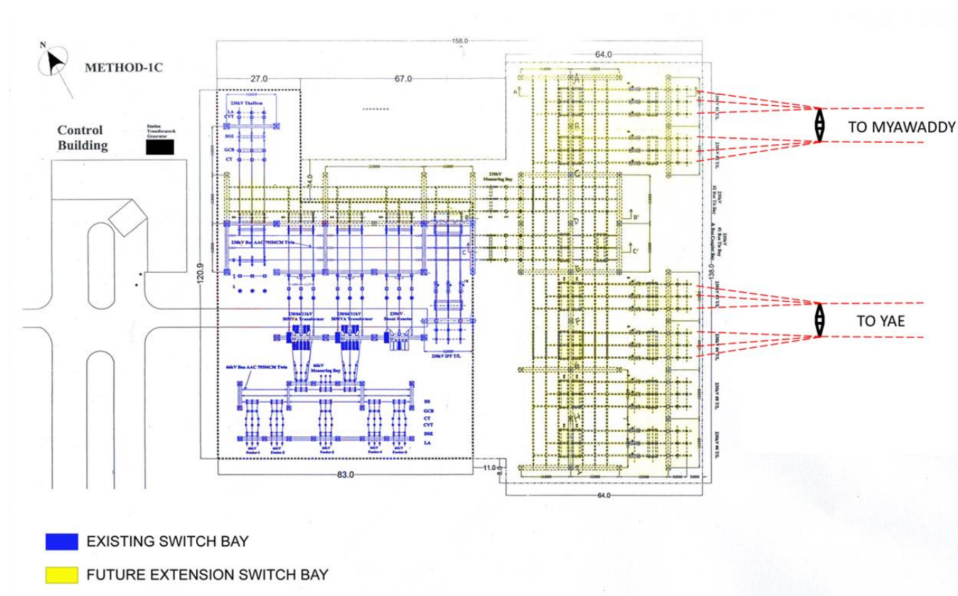
Figure 8: Layout of Existing Sub-Station at Mawlamyine, with future extensions
