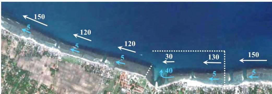
Figure E3. Annual Sediment budget at Point Pedro: unit –  $1000\text{m}^3/\text{year}$ , white arrows – sediment transport seaward of the reef, blue arrows – sediment transport between reef and the beach, white dashed lines represent the proposed harbour breakwaters (not included in model).
