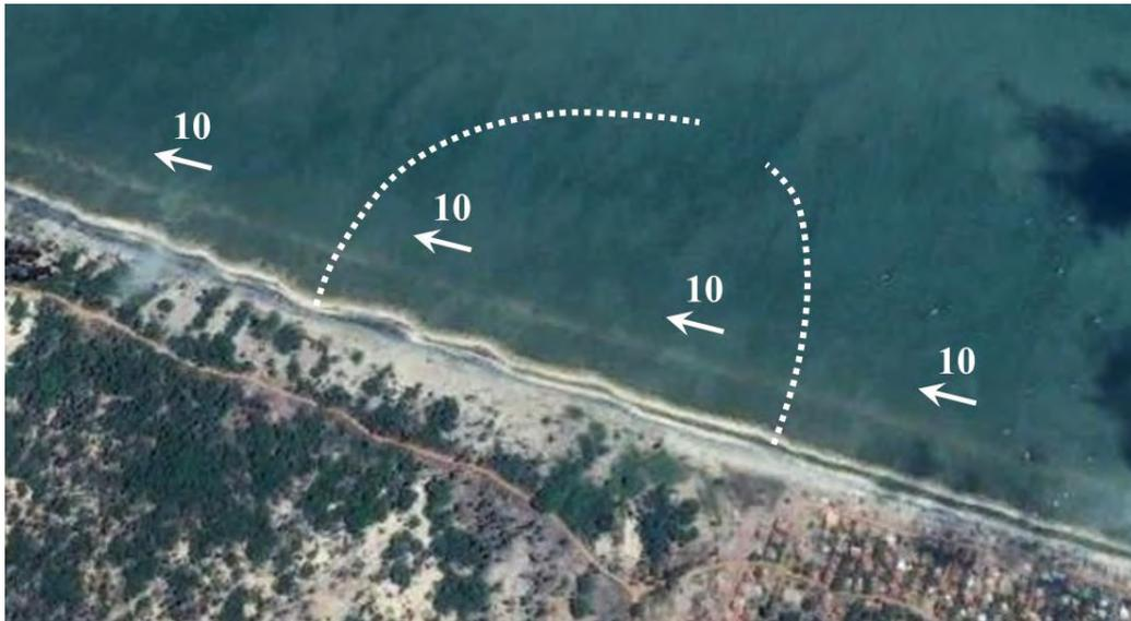
Figure 3.6 Sediment budget at Pesalai – white arrows, unit – 1000m<sup>3</sup>/year. White dashed lines represent the proposed harbour breakwaters which were not included in the model.
