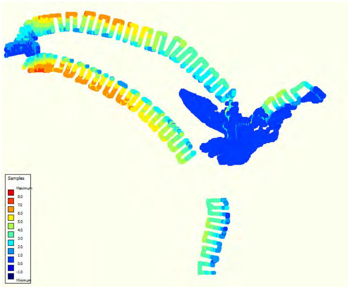
Figure 2.3 Mannar measured bathymetry (to MSL, downward positive)
