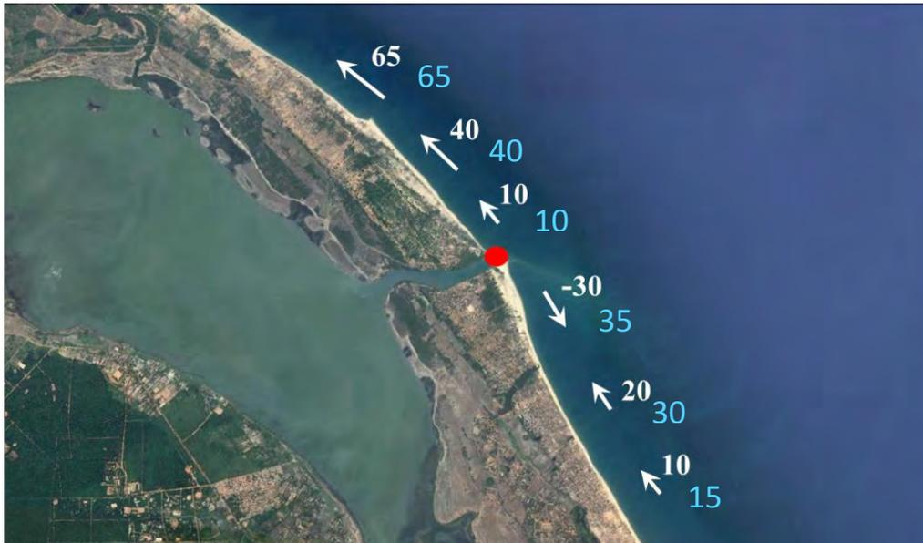
Figure 3.29 Sediment budget at Mullaitivu – white arrows and numbers show net longshore transport. Gross sediment transport rates are shown in blue numbers, unit – 1000m<sup>3</sup>/year. There is no layout of the proposed fishery harbour at Mullaitivu, the red circle shows the earlier proposed harbour location.
