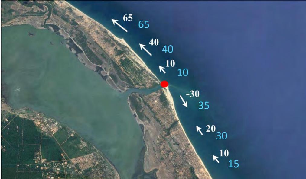
Figure E4. Sediment budget at Mullaitivu – white arrows and numbers show net longshore transport. Gross sediment transport rates are shown in blue numbers, unit – 1000m<sup>3</sup>/year. The red circle shows the earlier proposed harbour location.
