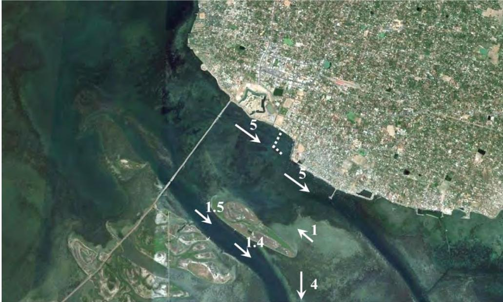
Figure 3.15 Sediment budget at Gurunagar - white arrows, unit 1000 m<sup>3</sup>/year. White dashed lines represent the proposed harbour breakwaters which were not included in the model
