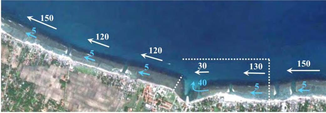
Figure 3.19 Sediment budget at Point Pedro: unit – 1000m<sup>3</sup>/year, white arrows – sediment transports behind the reefs, blue arrows – sediment transport between the reefs and the beach, white dashed lines represent the proposed harbour breakwaters which were not included in the model.
