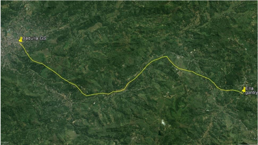
33 kV DC Lynx Tower Line from Badulla GS to Ella Gantry
