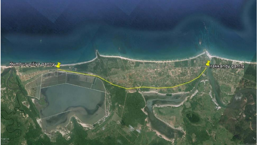
33 kV DC Lynx Tower Line from Irakkandy Gantry to Kumburupitiya Gantry
