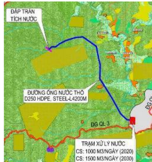
Basic design of water network including weir, main pipeline, water treatment plant
