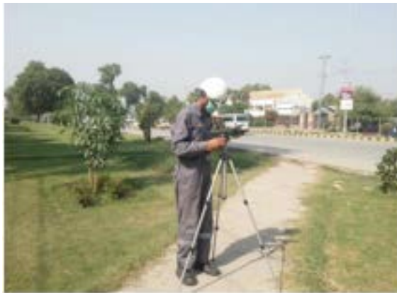
Photograph 11-1: SGS technician conducting ambient noise monitoring
