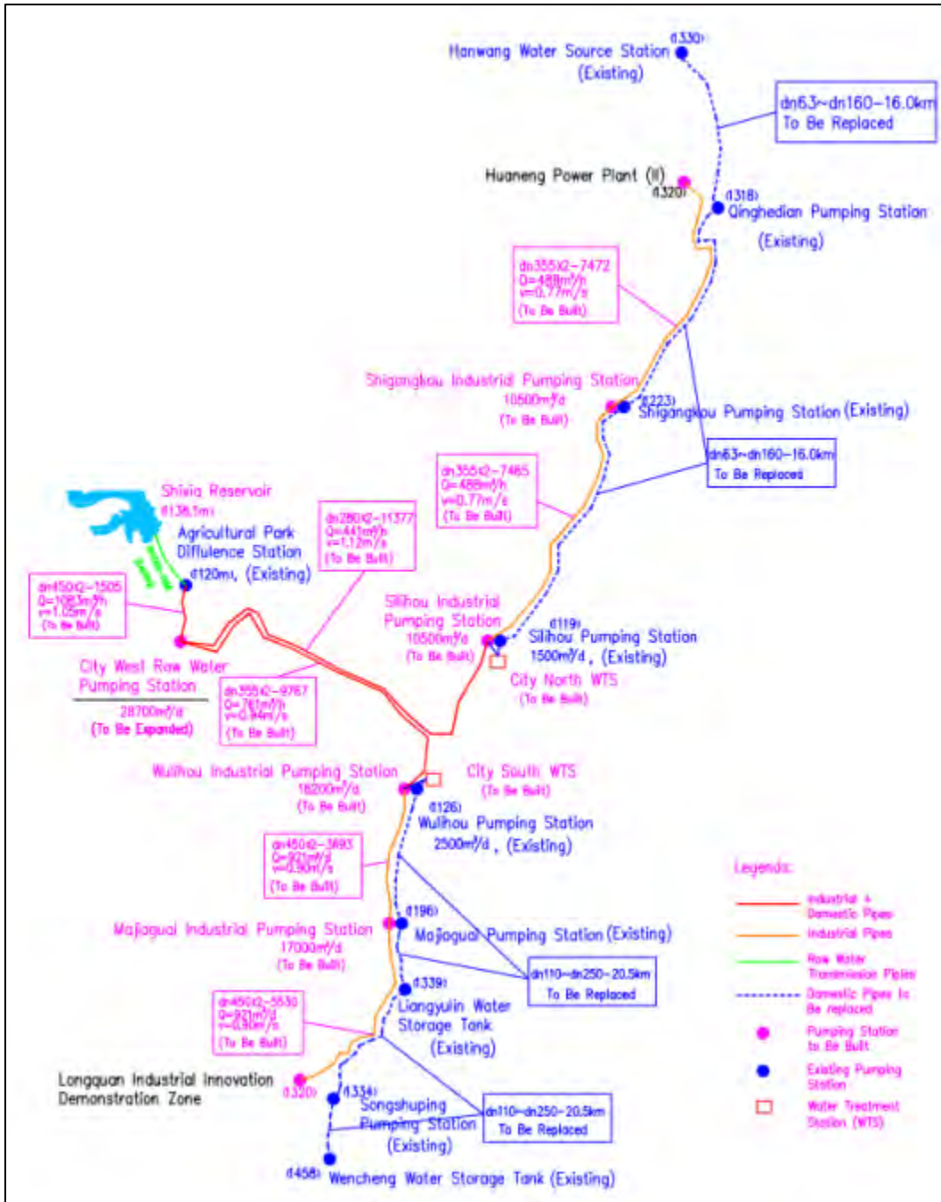
Figure IV-26. Layout of Water Supply System
