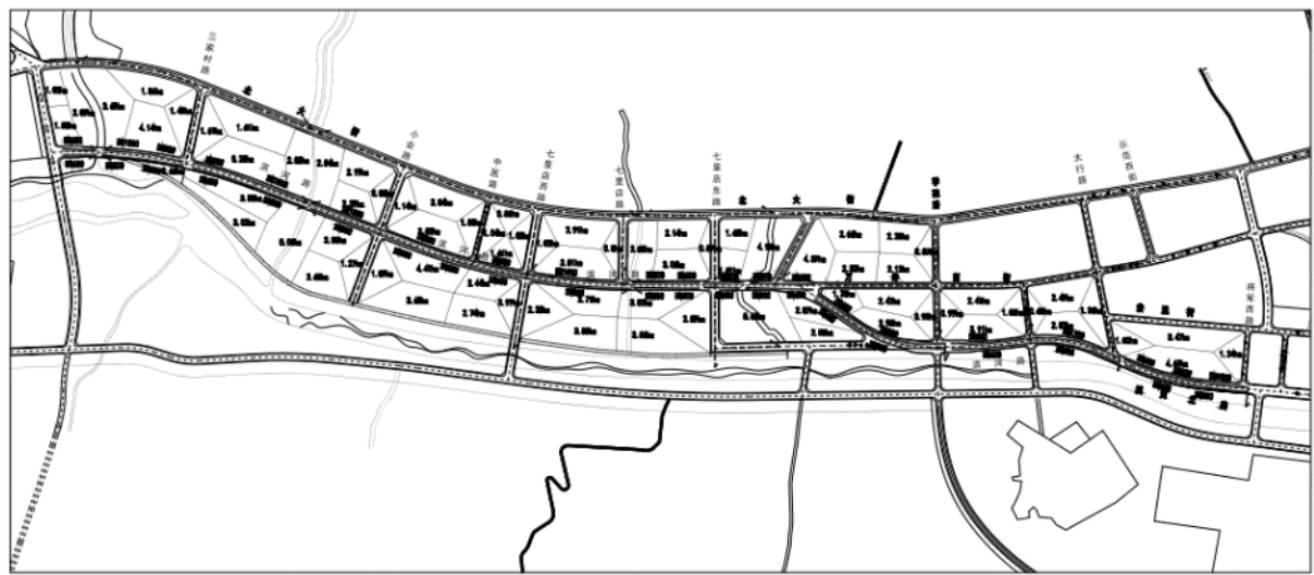
Figure IV-23. Stormwater Pipeline Layout
