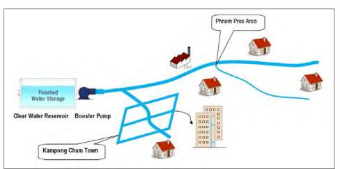
Figure 1: Option 1\_Schema of distribution pipe network (Pump only)
