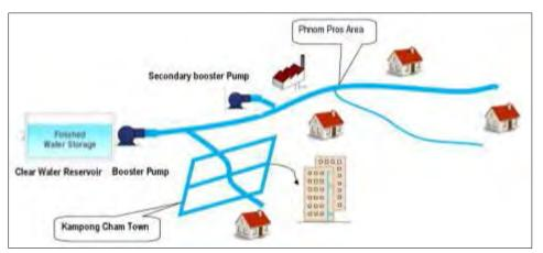
Figure 2: Option 2\_Schema of distribution pipe network (Pump +Pump)
