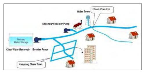
Figure 3: Option 3\_Schema of distribution pipe network (Pump +Pump + WT)
