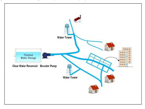
Figure 14. Network arrangements Option 1: booster pump with water tower
