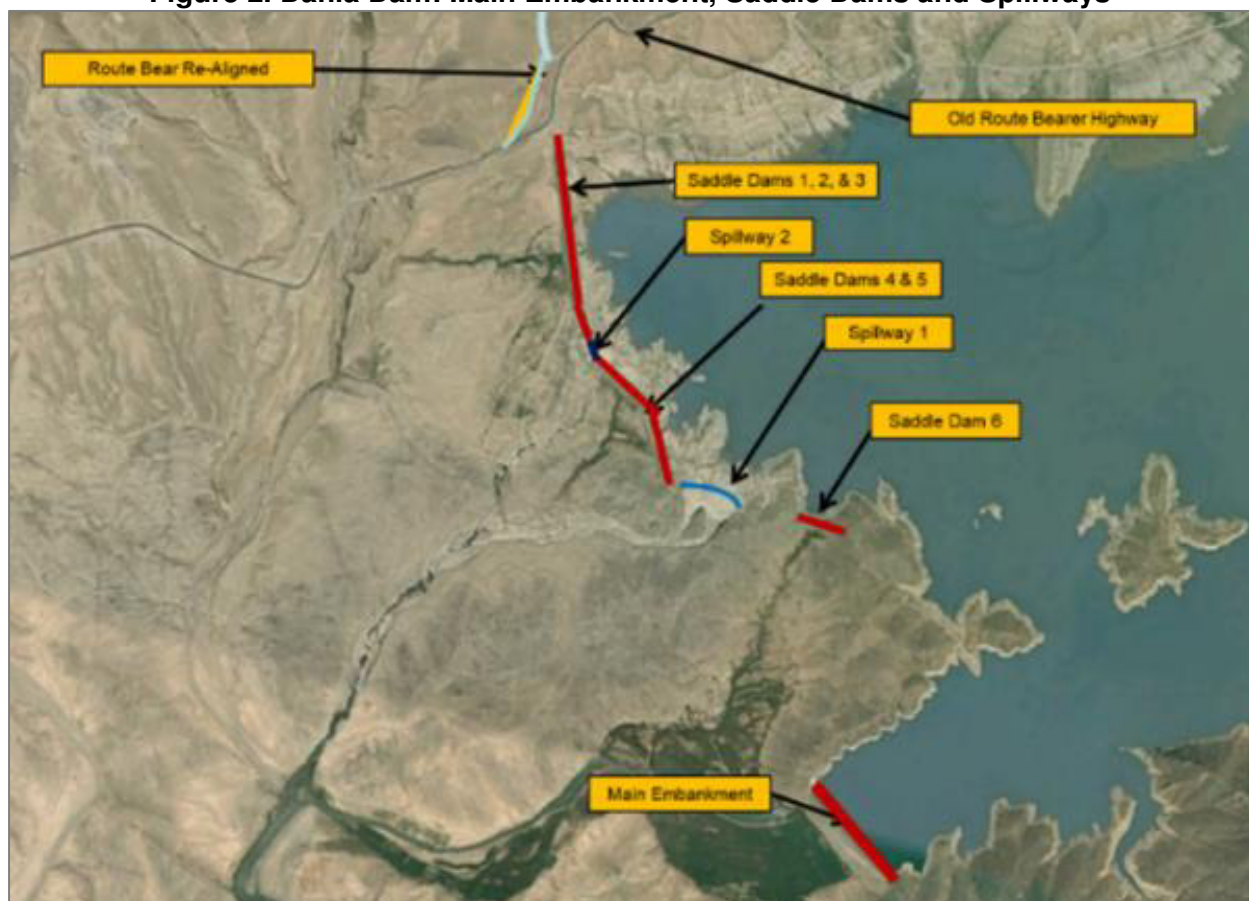
Figure 2. Dahla Dam: Main Embankment, Saddle Dams and Spillways
