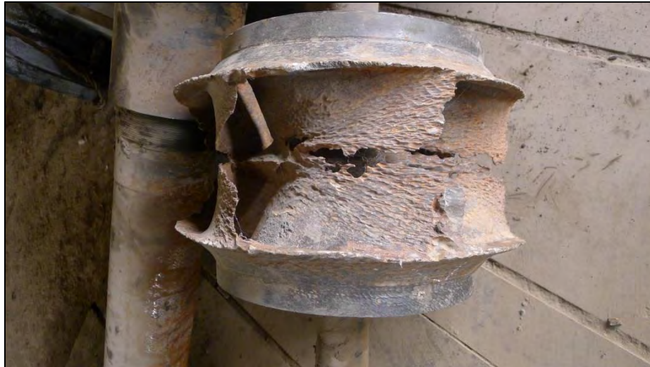
Figure 11: Heavily Damaged Pump Impeller
