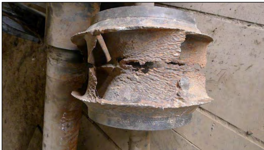
Figure 11: Heavily Damaged Pump Impeller
