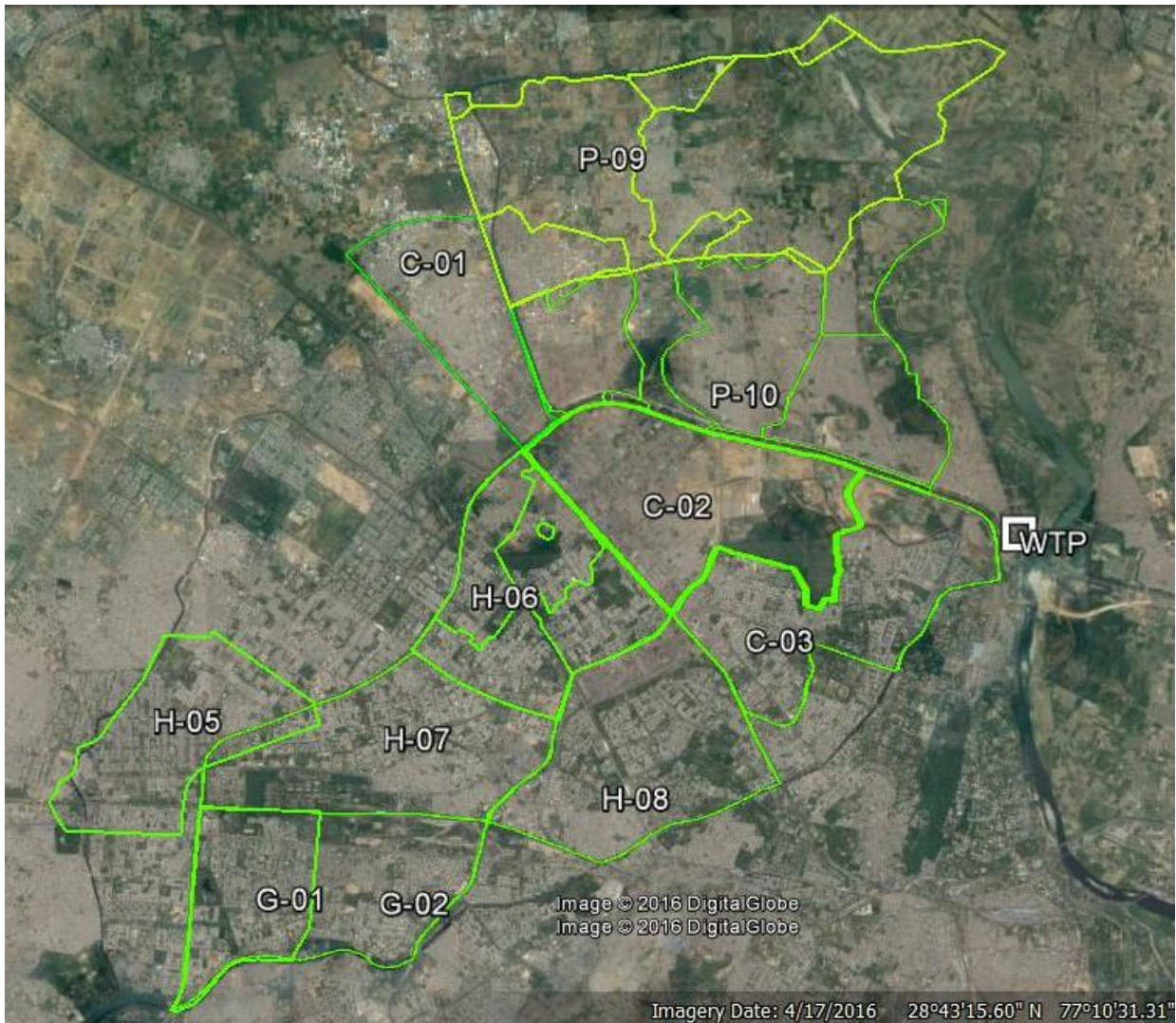
Figure 2: Underground Reservoir Command Areas & WTP
