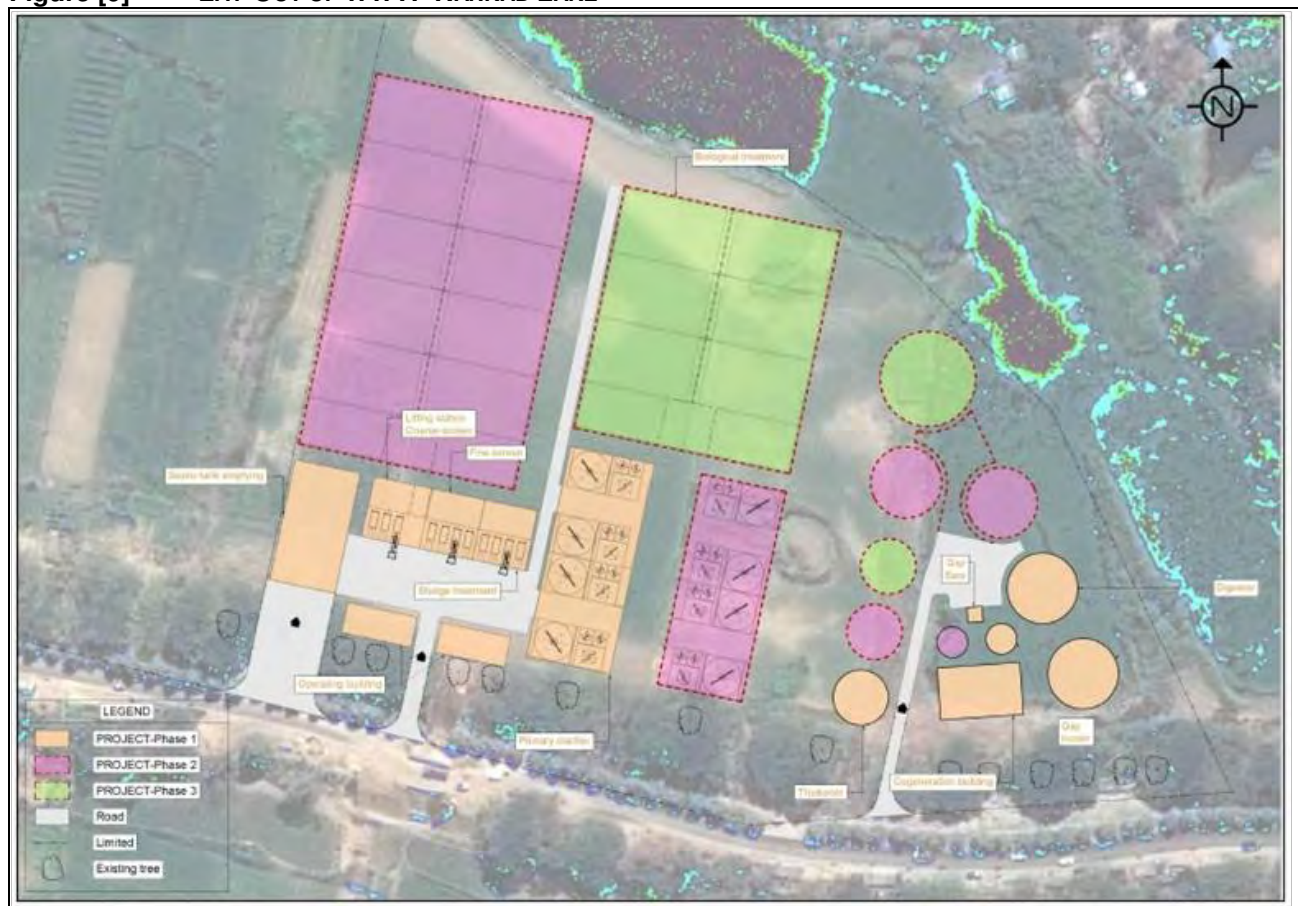
Figure [9] LAY-OUT OF WWTP NANKAD LAKE
