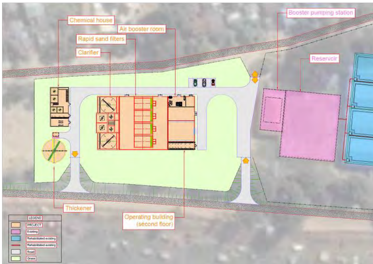
Figure [4] SITE LAYOUT OF WTP N° 8 EXTENSION
