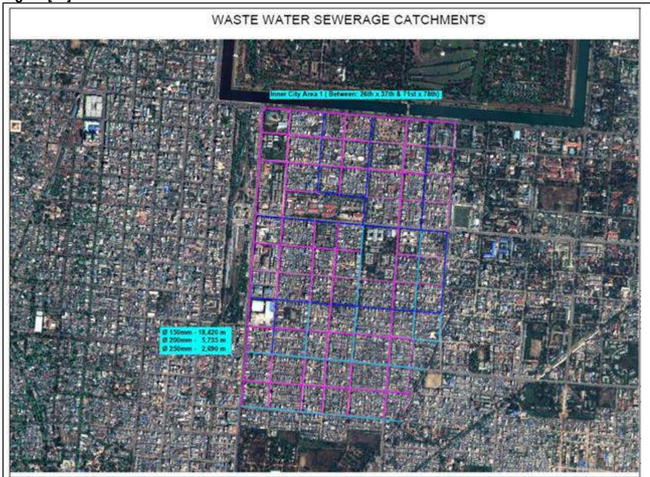
Figure [11] PROPOSED PILOT PROJECT AREA WITH RETICULATION SEWERS
