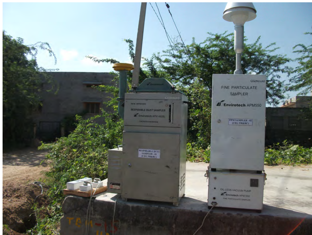
Figure 4.5 : RDS APM 460 BL and Fine Particulate Sampler APM 550
