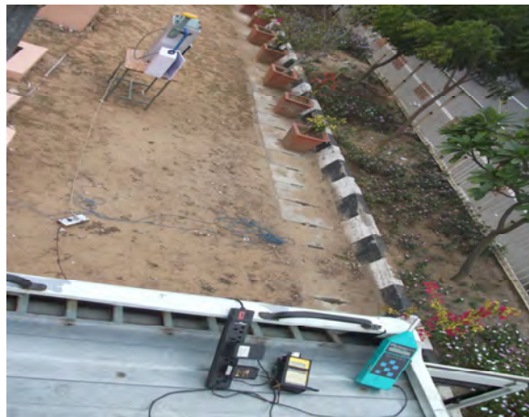
Figure 4.6 : SLM 100 (Monitoring of Noise Level) Rania km 447
