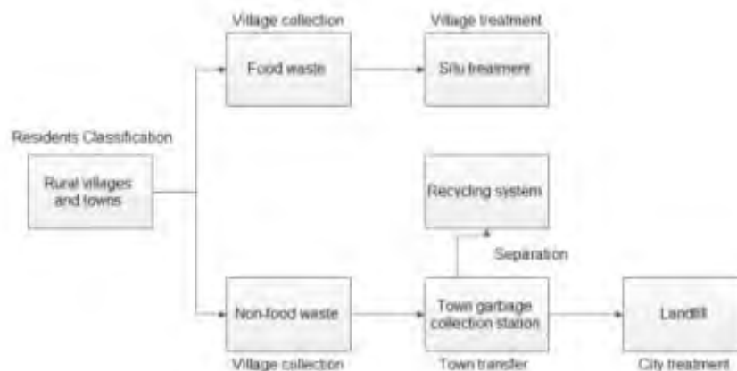
Figure IV-7: Solid waste collection and treatment flow diagram
