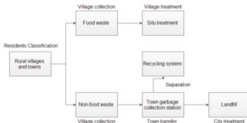
Figure IV-7: Solid waste collection and treatment flow diagram
