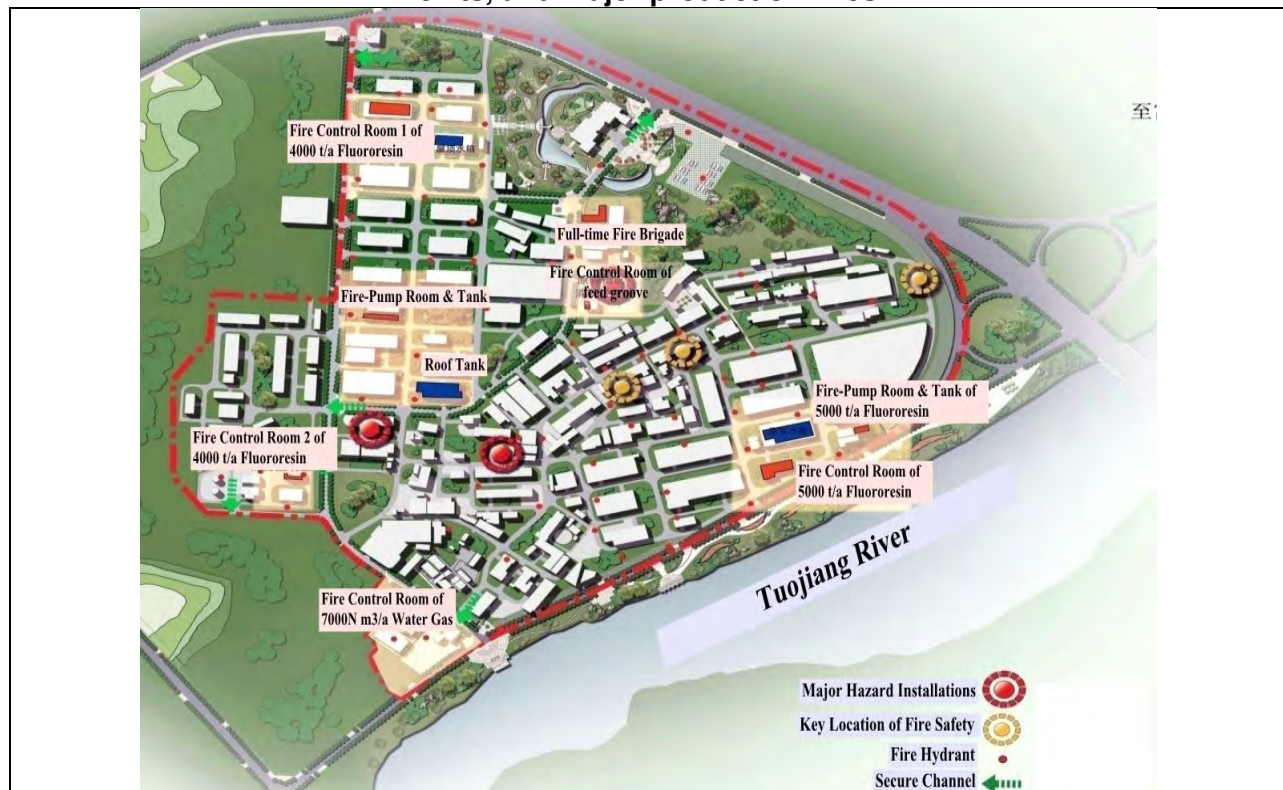
Figure 6. CGY plant layout with indication of major hazards, fire hydrant, emergency exits, and major production lines
