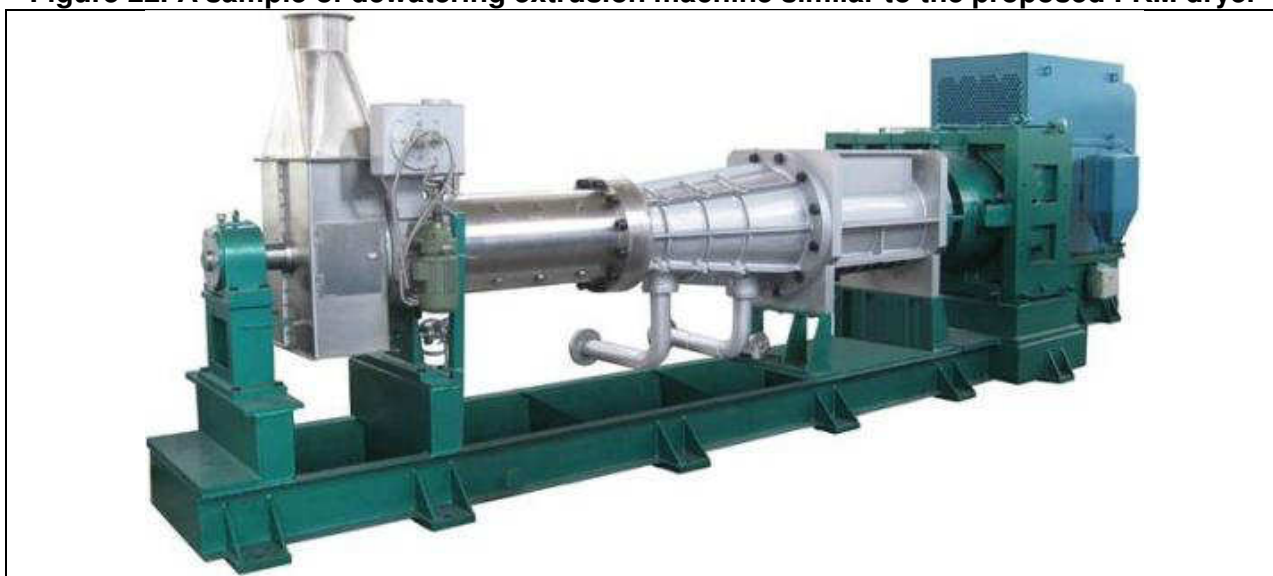
Figure 22. A sample of dewatering extrusion machine similar to the proposed FKM dryer
