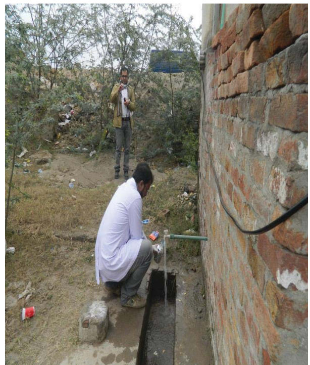
Fig32: Ground Water Sampling
