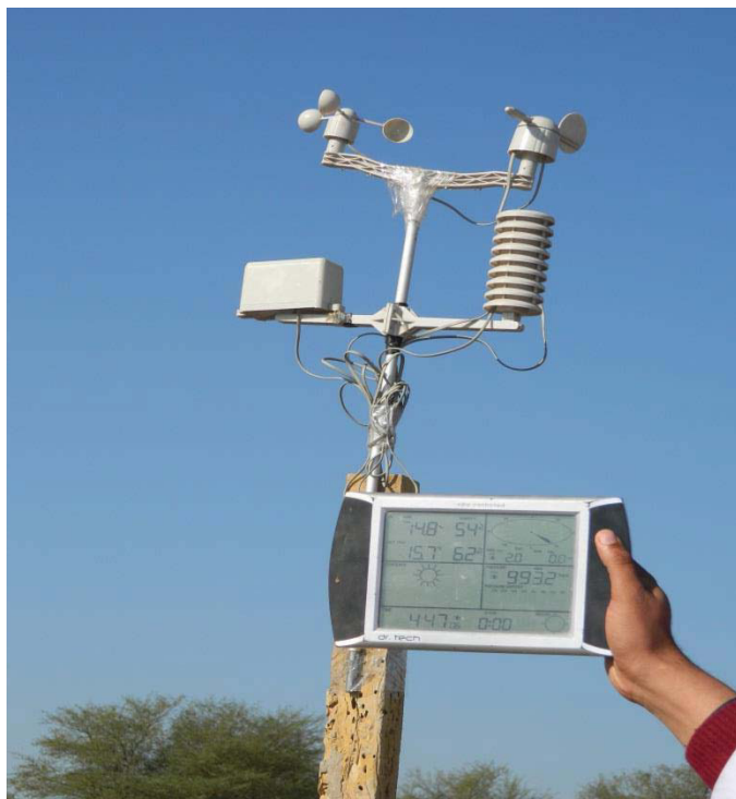
Fig31: Weather Station Monitoring at Pind Dadan Khan Site
