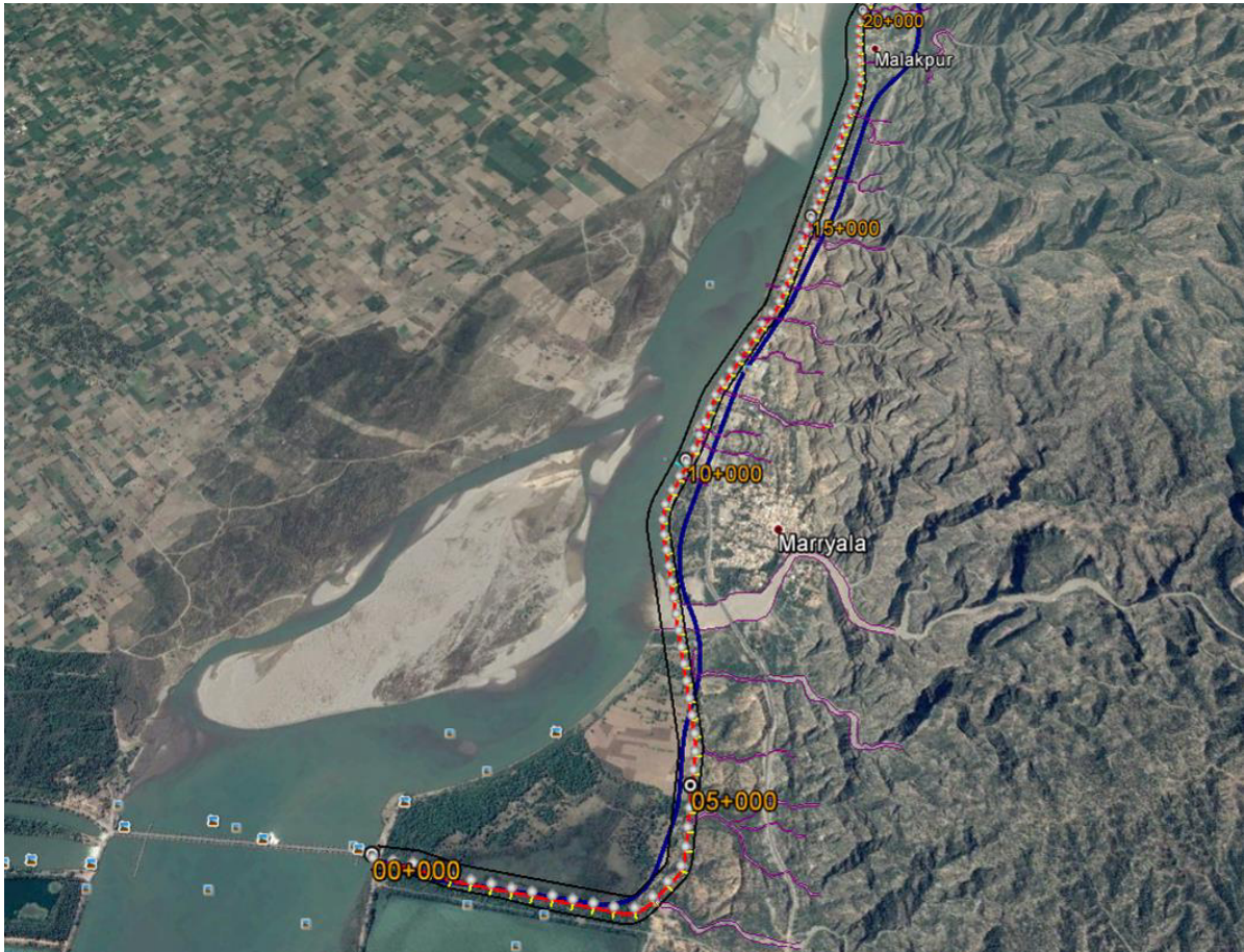
Figure 5.4: Main canal Alignment RD 0+000 to RD 19+000
