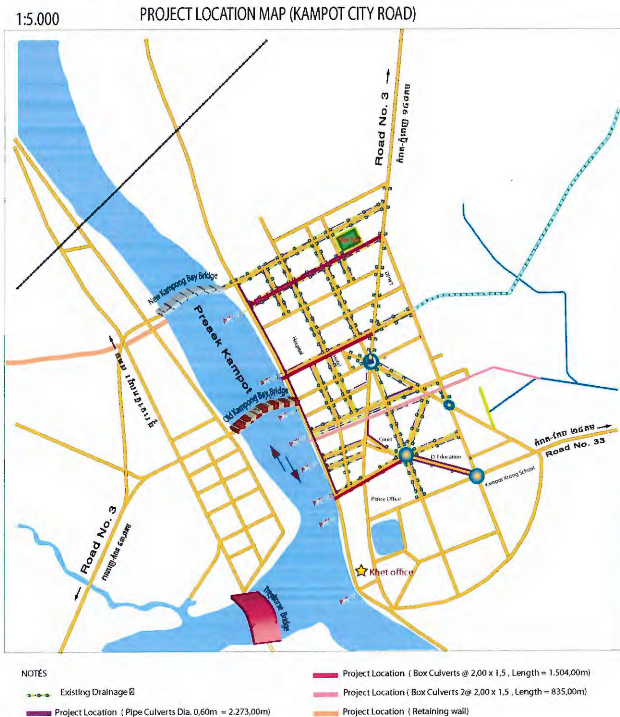
Figure 7. Locations of drainage network to be upgraded in Kampot.
