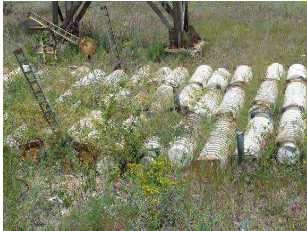
Photo 4-14: Ceramic waste stored at a substation site
