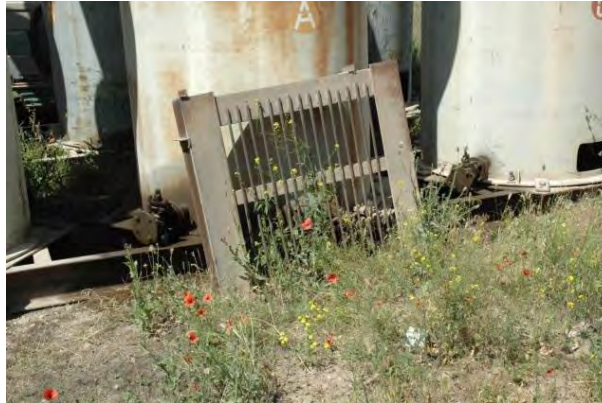
Photo 9-2: Discarded equipment is used for storage of old and/or spare oil. This old equipment is often leaking.
