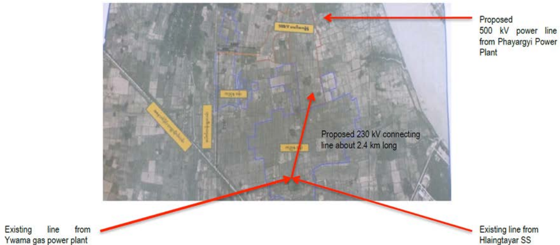
Figure 2: Layout of the Proposed West University Substation
