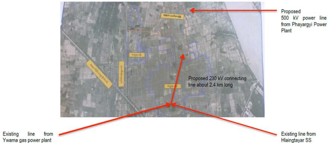
Figure 2: Layout of the Proposed West University Substation
