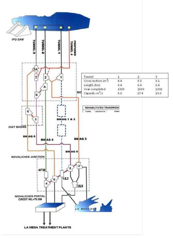
Figure 1: Schematic layout of transmission system
