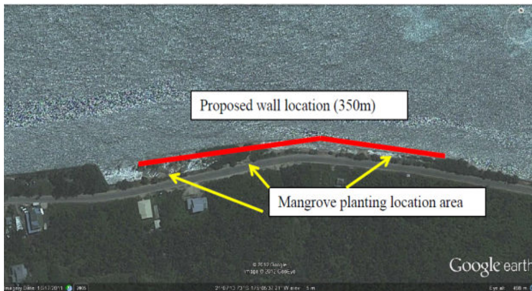
Figure 19: Proposed intervention for seawall rehabilitation and mangrove planting and rehabilitation
